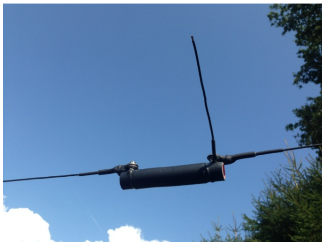
Figure 5: Piece of wire at the output of the 1st extension spool
